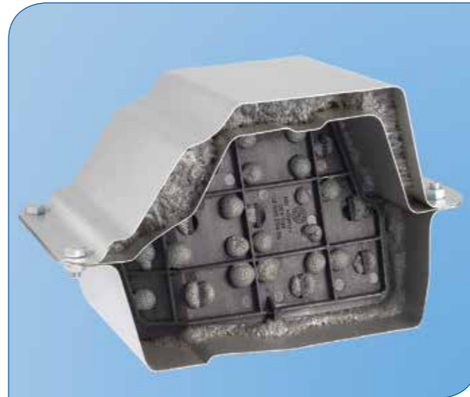
L&L Seal heat-expandable, baffle systems reduce cavity borne noise within the vehicle structure. They are available in a range of forms, expansion rates and cure temperatures to suit build rates, design and geometry requirements and curing processes.
