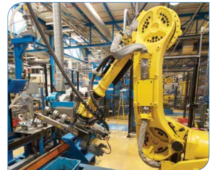
Robotic application of XiP Extrude-in-Place sealants and adhesives
