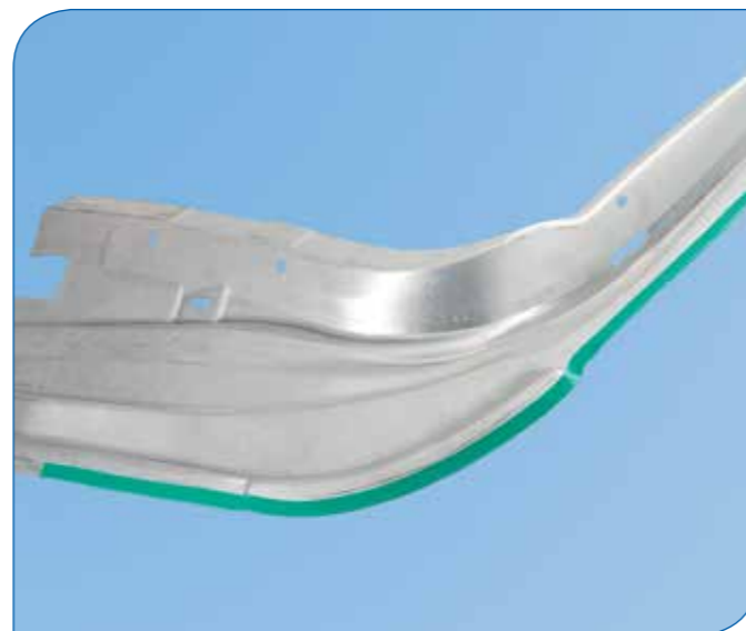
L&L Bond and L&L Seal XiP systems are heat expandable adhesive and sealing systems for a range of anti-flutter, sealing, anti corrosion and bonding applications. As they are dry to touch materials, 'adhesive wash out' problems are eliminated.
